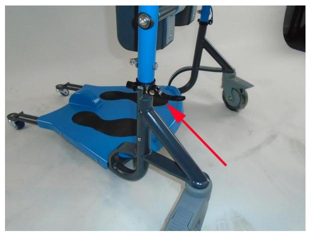
2. Raise or lower the upper half of the unit according to the height required. There are two stop points with spring pins setting the lowest or highest points. The height of the upper half can be set anywhere between the lowest & the highest point. (See photo below)
